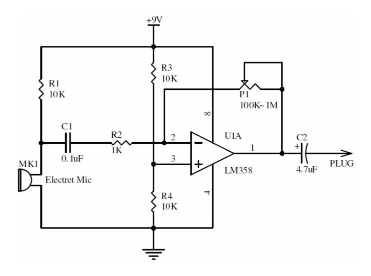
This circuit will be useful if you have an electret microphone that produces a low audio (sound) level and you want to connect it to an amplifier or something like it. The circuit will boost the microphone output voltage to obtain an acceptable signal level. Just adjust the R5 potentiometer to obtain the desird gain. Note that the R5 value is dependent on your gain need.
